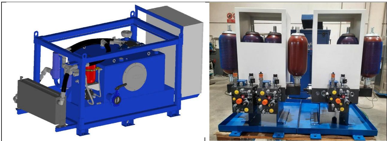
Figure 1: Silence HPU and HSM Manifold
